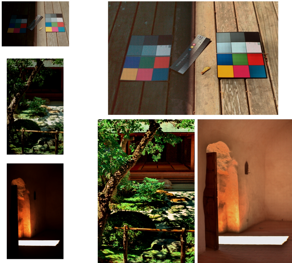
Figure 4 shows three pairs of images. The left column has small unprocessed control images. Here digits are proportional to log radiance in the scene. These images were printed normally. Note that the test target in the sun appears normal. The same test target in the shade is much darker. The larger Retinex images on the right have been spatially processed to compress the dynamic range of the image then scaled to fit the printer dynamic range. Again, the output images are not colorimetric reproductions, rather they preserve the edge information and the relationships of all parts of the image.
