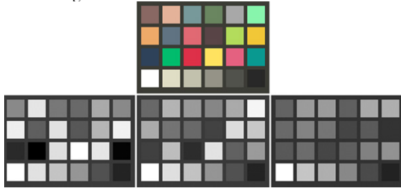
Figure 4 (top) shows the digital color image selected by observer matching session for tungsten light; (bottom) show the digital R, G, B separation images used in making the color image on the display. The colors chosen here have different color separation images. It is important to note that the colors seen on the printed page do not have the same appearance as those in the viewing booth. These images illustrate the digital values of the matches.
