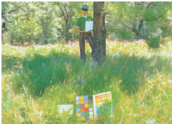
Figure 5 shows an example of an HDR scene processed with spatial comparisons. (1978 Frankle and McCann patent application). The illumination on the white card in the shadow is 1/32^{\text{th}} that on the black square in the sun. Both the white card in shade and black square in sun have the same luminance. The spatial processing converted equal input digits ( -\log luminance) into very different output digits, thus rendering the HDR scene into the small range of the reflective print shown here.
