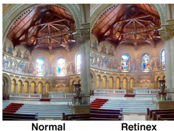
Figure 8 shows images with and without spatial comparisons, both taken with a commercial HP 945 camera. The pictures are hand-held single-exposure images. The image on the right uses Retinex based Adaptive Lighting/Digital Flash camera options. The spatial processing removes the over-exposure of the windows while lightening the red rug, white marble altar and pews.
